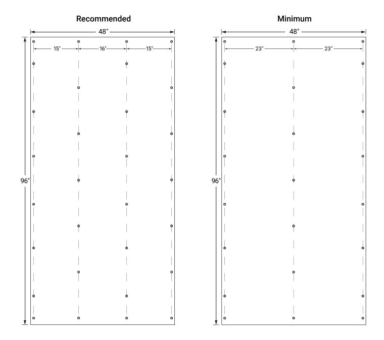
Drainwall Panel Fastener Layout
