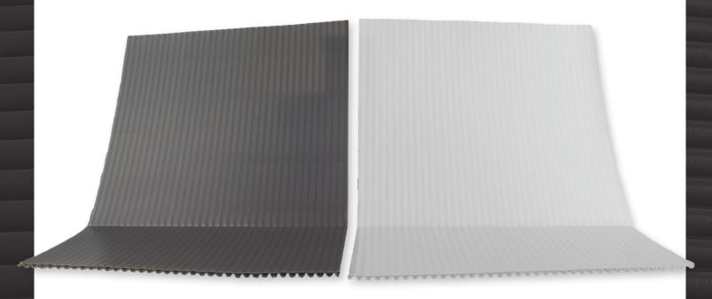
Richtech's Channel-Cove is a seamless water diverter that keeps water in the drain and off the basement floor. Fluted channels collect water from the wall and weep holes and direct it under the floor into any sub-floor drain system. The smooth white facing is attractive and can be trimmed with Channel-Cove cap molding for a clean, professional finish.
